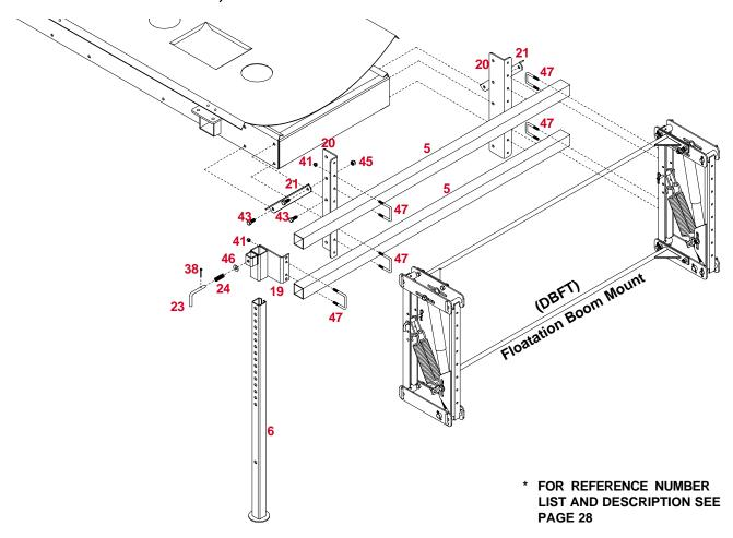
NOTE: Always lock the Safety Stand in the down position when unhitching the sprayer and lock it in the up position before towing the sprayer.
